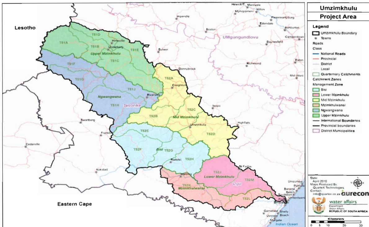
Figure 1: Project Area, showing the Quaternary sub-catchments and the six Water Management Sub-catchments
